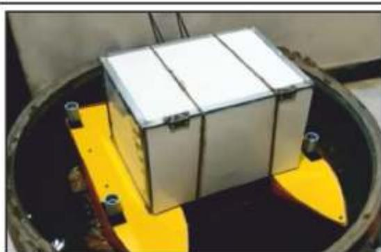
Static Buoyancy Testing of the prototype
