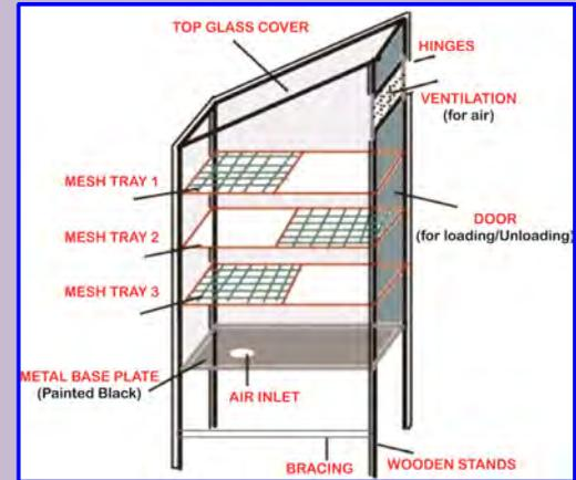
Schematic Layout of Mini Solar Dehydrator
