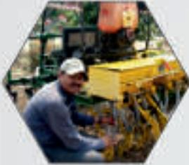
Seed sowing and fertilizer dropping attachments for all types food-grains at 9-11 inch crop lane distance
